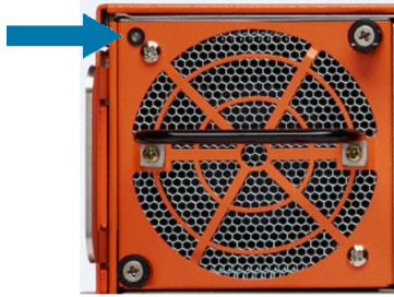
Figure 6 Individual Fan LED Location on GigaVUE-HC3 Rear
